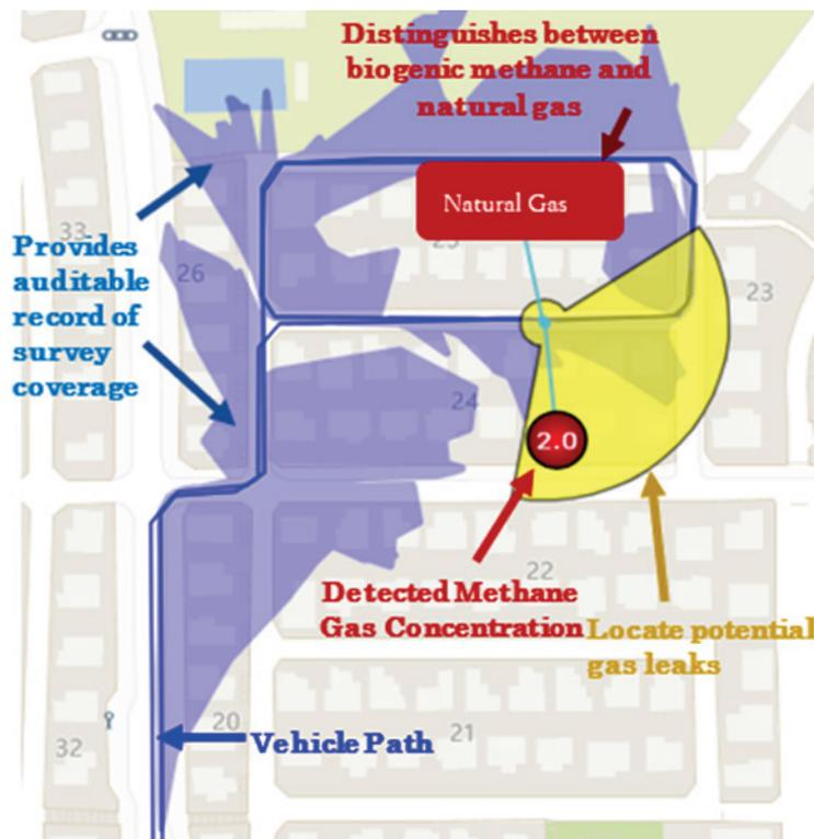
Figure 2 Example of Inspection Results Displayed in P-Cubed
