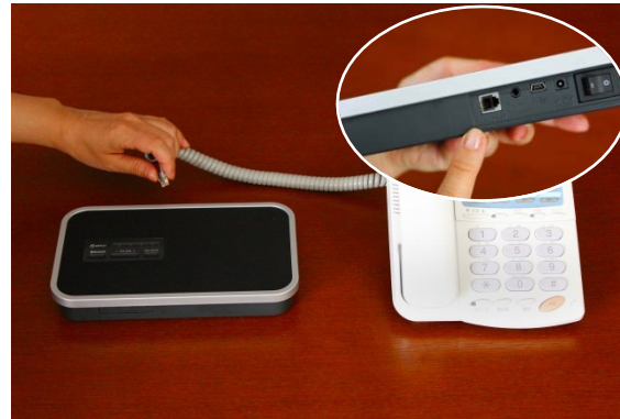
2 Insert the coiled cable into the handset cable outlet of the R-Talk 800EX
