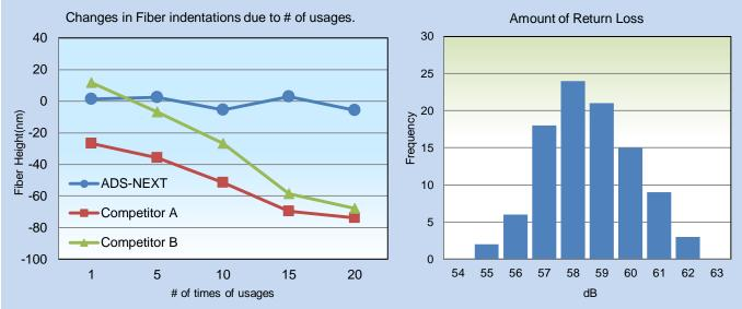
%This data is an example of polishing results. Results are influenced by various factors, such as polishing conditions, the polisher used, and the type of ferrule.
