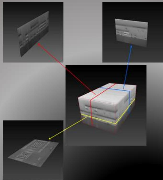
Step1 FIB slightly process and observe the exposed cross section with SEM
