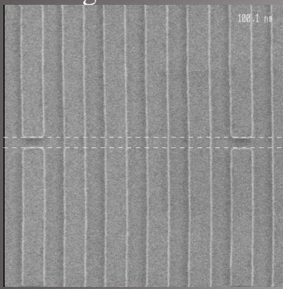
SEM image of L&S with isolation thin line width
