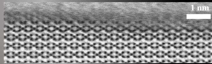
STEM image of sapphire substrate surface (R-plane)
